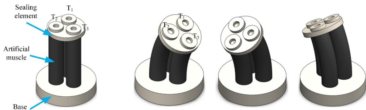
Fig. 5. Simplified Model of the Flexible Robot and Its Presentation of Motion
