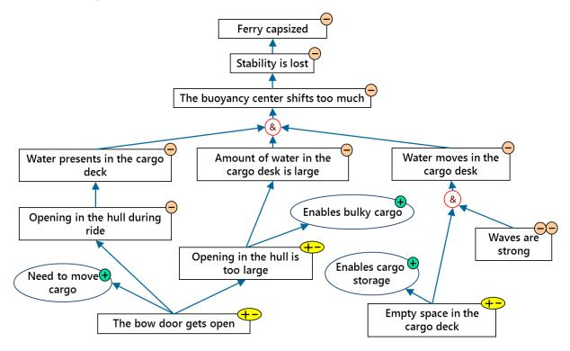
Note, that to eliminate a general negative effect "Ferry capsized" in order to prevent the reoccurrence of that specific situation, it would be enough to eliminate any single cause presented in the diagram. It is possible because all causes and branches of the RCA+ tree are connected through "AND" relationships.
