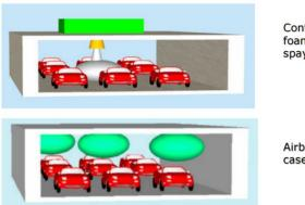
Containers with liquid plastic foam which solidifies after being spayed in case of emergency
