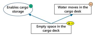
A physical conflict can be formed on the basis of this triad as follows: "Open space must be in a cargo bay to enable loading/uploading of bulky cargo and must not be there in order to avoid movement of water during an accident".
