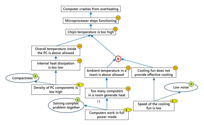
After the RCA+ model of a problem is completed, a table of revealed problems is created, and selection of a particular conflict to solve is made on the basis of the desired changes in the system.
