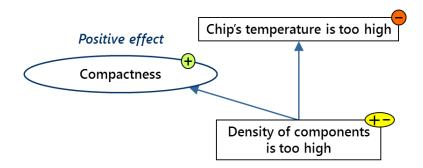
At this diagram, we can see that while the high density of components in a computer is positive to provide compactness, at the same time it is also negative since it produces overheating of the microprocessor chip. Such a "triad" model gives us a direct indication of both technical and physical contradictions which are present in the system:
